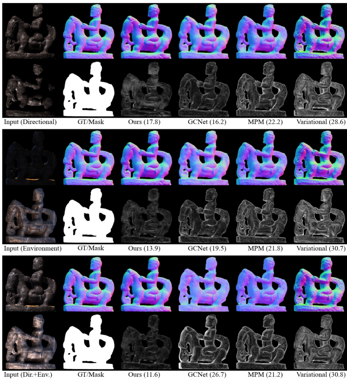
Figure 42. Results on object ID 40 (statue-2, tiling-42 [Floor]). MAEs (in degrees) are shown next to the name of the method.
